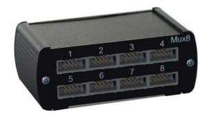
This range offers the possibility to connect most of the control instruments of the market (micrometers, calipers, weight scale etc...) and is divided into 4 products for connecting respectively 2, 4, 8 or 16 instruments on a PC.
