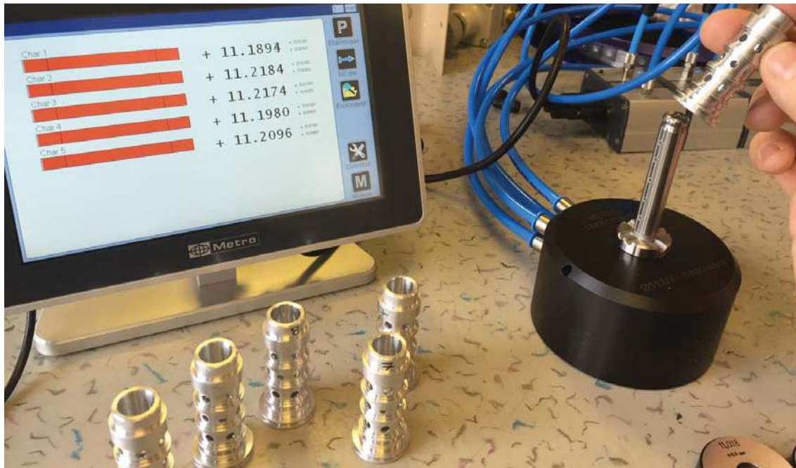
5 levels air gage connected on the M400 through 5*MB-AG modules
