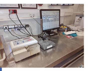
This control system is used to check several dimensions on connecting rods using air gaget. Several parameters are checked, including internal diameters, bend and twist. The measurements are temperaturecompensated.
